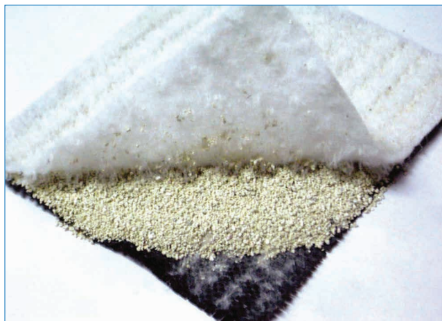
Figure 6. Geosynthetic clay liners
