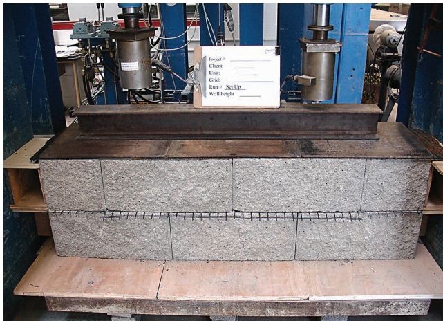
Figure 19. Geogrid connection testing with SRW units
