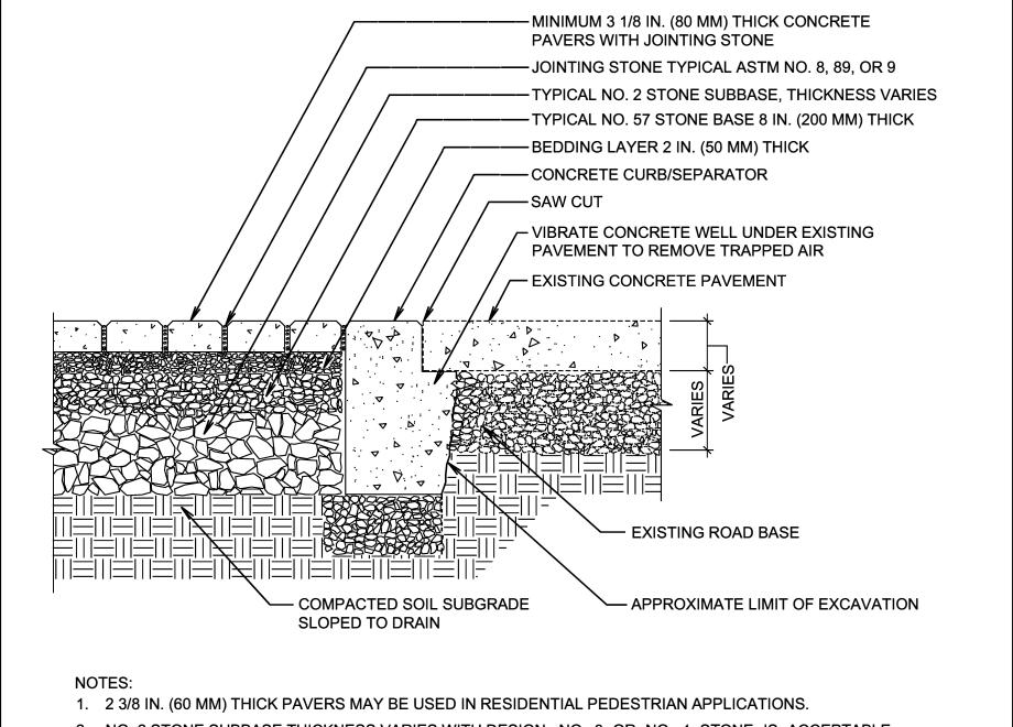
2. NO. 2 STONE SUBBASE THICKNESS VARIES WITH DESIGN. NO. 3 OR NO. 4 STONE IS ACCEPTABLE. CONSULT ICPI PERMEABLE INTERLOCKING CONCRETE PAVEMENT MANUAL OR ASCE 68 18.
