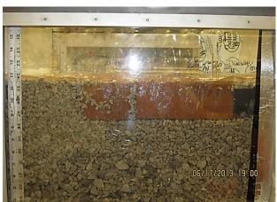
Top left and right: Flume containing PICP measures surface and subsurface flows and volumes. Bottom left and right: PICP surface at the flume end and cross section with jointing, bedding and No. 57 stone base.
