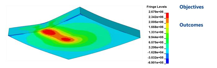
Finite element modeling illustrates the principal stresses in megapascals (MPa) on the bottom surface of 48 x 48 x 4-inch thick paving slab subject to a dual truck wheel load. (To convert MPa to psi, multiply by 145.)
