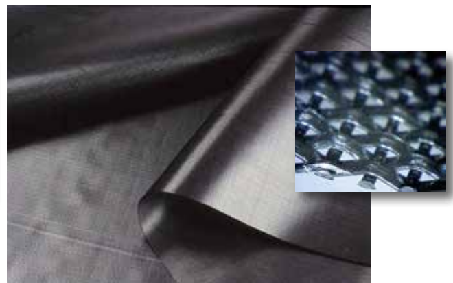
Figure 12. Woven mono-filament geotextile with close-up
