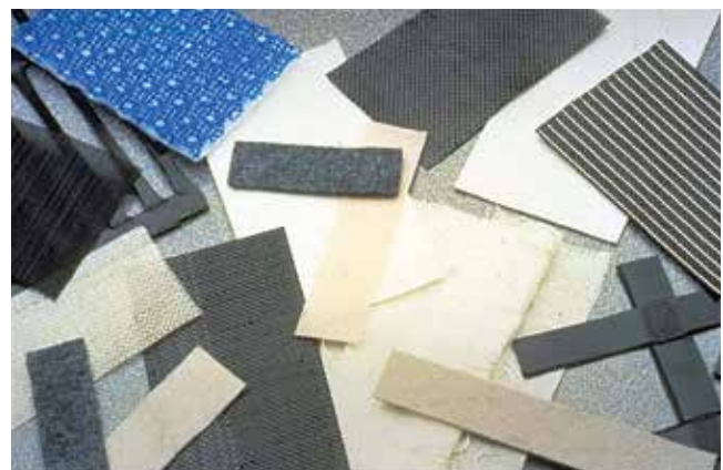
Figure 1. Different types of geosynthetics
