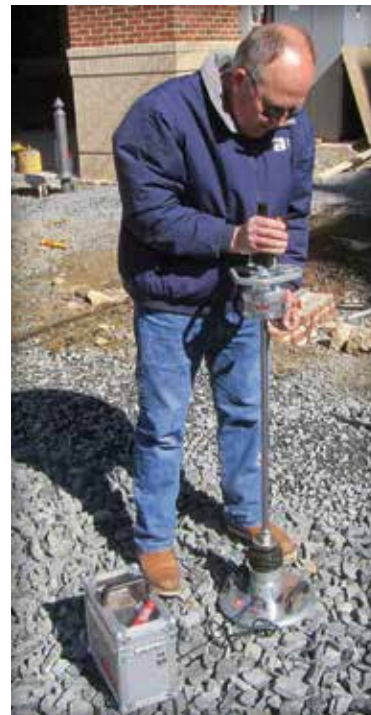
Figure 22. Testing base stiffness using light-weight deflectometer.
