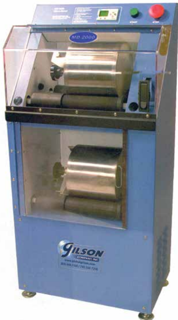
Figure 1. The Micro-Deval test apparatus. Source: Gilson Company
