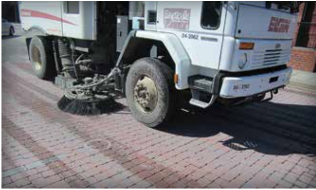
Figure 21. A regenerative air machine does routine cleaning in a PICP parking lot.
