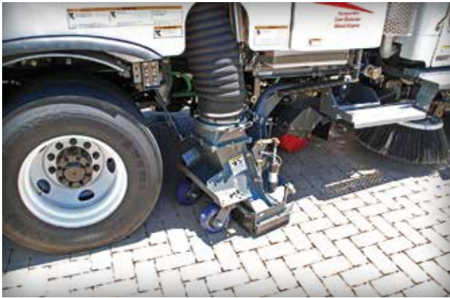
Figure 22. A true vacuum machine cleaning neglected PICP.
