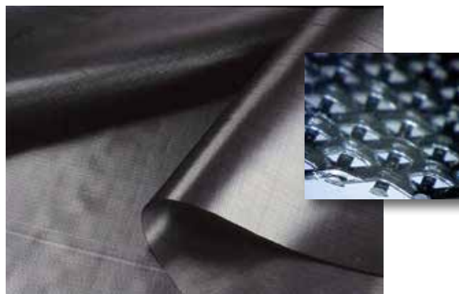
Figure 12. Woven mono-filament geotextile with close-up
