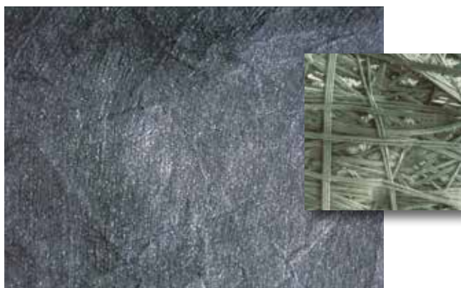
Figure 15. Non-woven heat bonded geotextile with close-up
