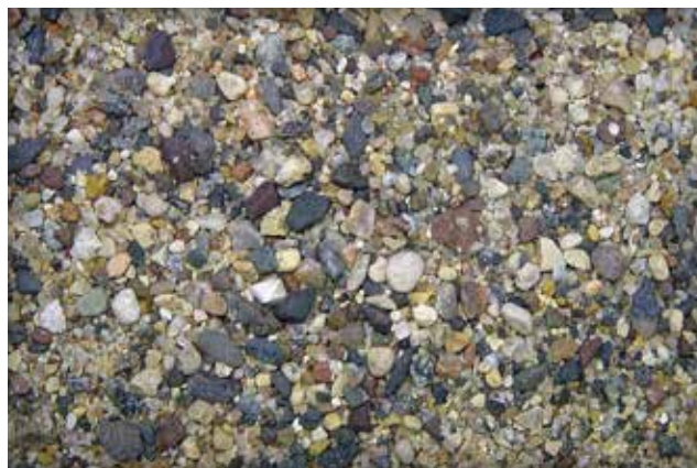
Figure 3. Example of sand from the ICPI bedding sand test program with a total combined percentage of sub-angular and sub-rounded particles equal to 65% according to ASTM D2488
