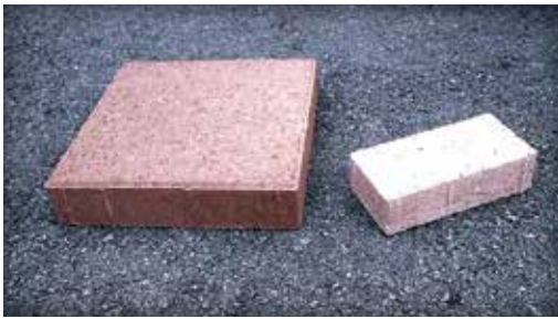
Figure 3. Concrete paver (right) and a concrete paving slab (left): similar paving products with varying applications for roof decks.
