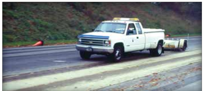
Figure 5. ASTM E274 Test Equipment consists of a truck and trailer assembly. A tire within the trailer is towed at a given speed, locked, and skidded across water dispensed on the pavement in front of it.
